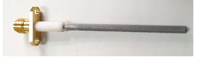
Fig. 3. Close-up of connector and outer resonator assembly, after press fitting.
