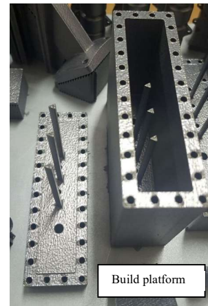
Fig. 2. Interdigital filter, using triangular bars, placement on build platform.
