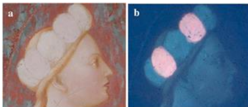
Figure 2.6: Fluorescence of Salome's face painted by Masolino di Panicale. a) Visual image; b) UV-induced fluorescence excited at 365 nm with an UV-A low pressure mercury lamp [16].
