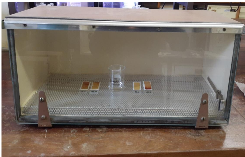
Figure 3.3: A photo of the chamber which was saturated with ammonia vapour from a 25% ammonia solution.
