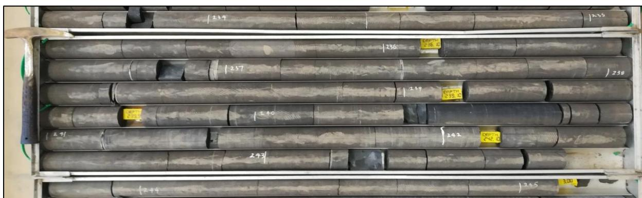
Figure 17: KZF-01 Fine sandstone in the core box
