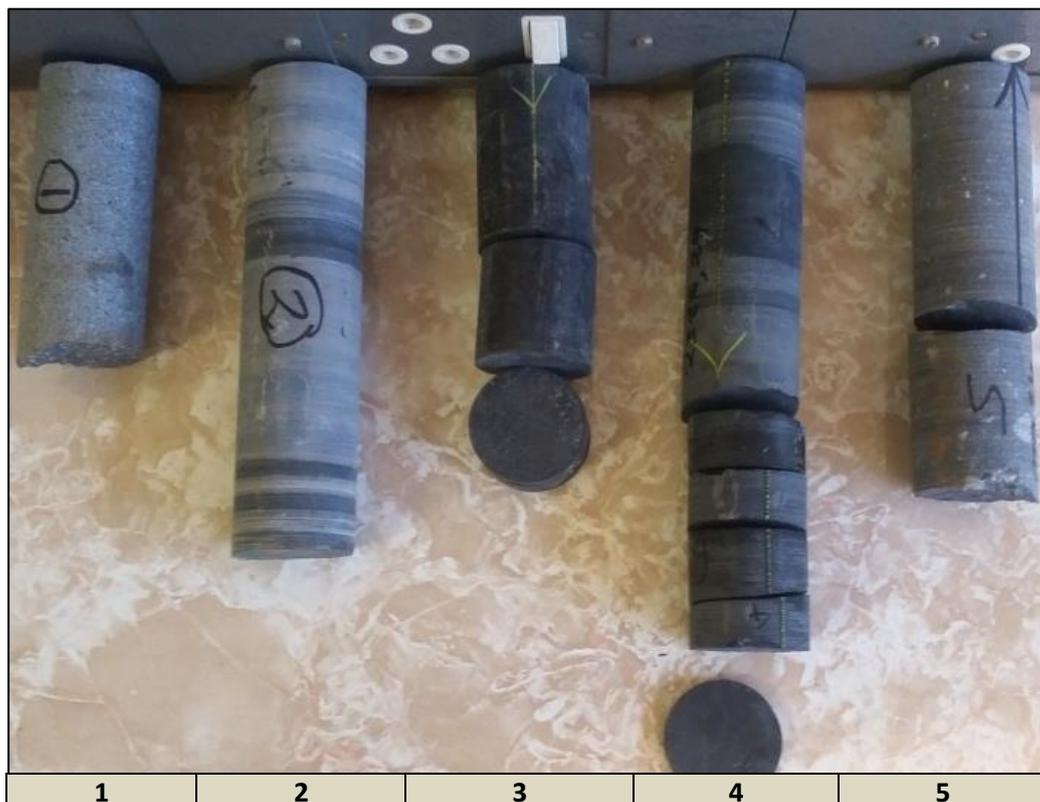
Figure 10: Five representative core samples taken from the borehole KWV-01. (From left to right - dolerite, sandstone, carbonaceous shale, massive shale and tillite)
