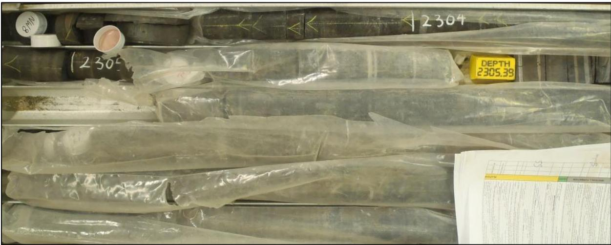
Figure 13: KWV-01 Carbonaceous shale individually wrapped in plastic bags in the core box
