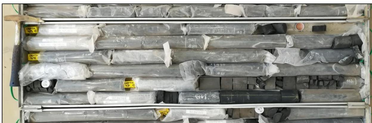
Figure 18: KZF-01 Carbonaceous shale in the core box
