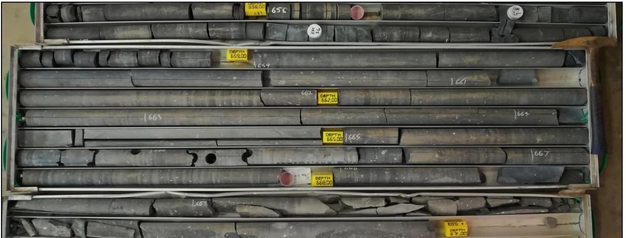
**Figure 20: KZF-01 Diamictite retrieved in the second last core box of the borehole KZF-01**
