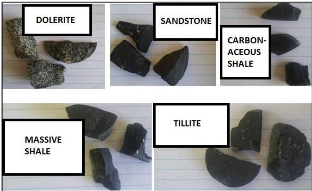
Figure 25: KWV-01 Oven-dried samples before Ethylene Glycol Soaking Test
