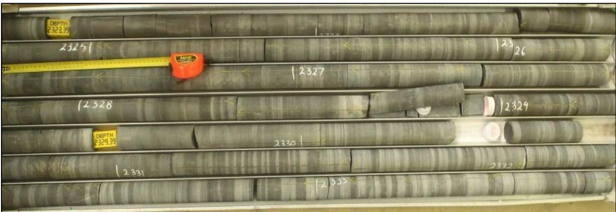
Figure 14: KWV-01 Massive shale in the core box
