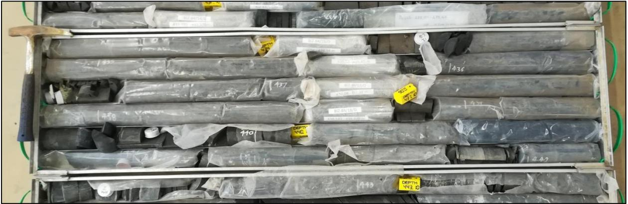
**Figure 19: KZF-01 Shale in the core box**
