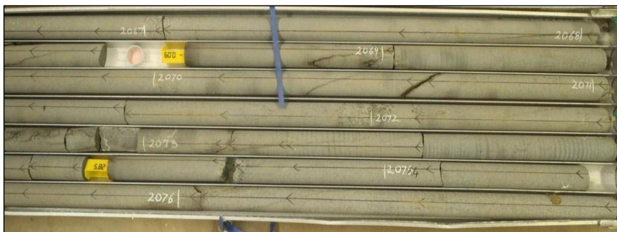
**Figure 11: KWV-01 Dolerite in the core box**
