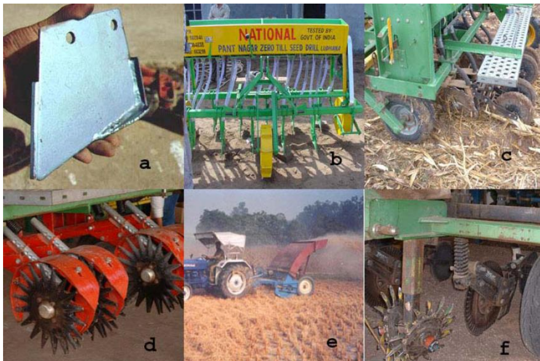
Figure 2.2 Equipment for planting in no-till. (a) inverted-t coulter; (b) Indian no-tillage drill using inverted t; (c) disk type planter; (d) star-wheel punch planter; (e) “happy planter”, which picks up straw and blows it behind the seeder; (f) disk plants straw and blows it behind the seeder (Source: http://www.ecaf.org/index.php )
