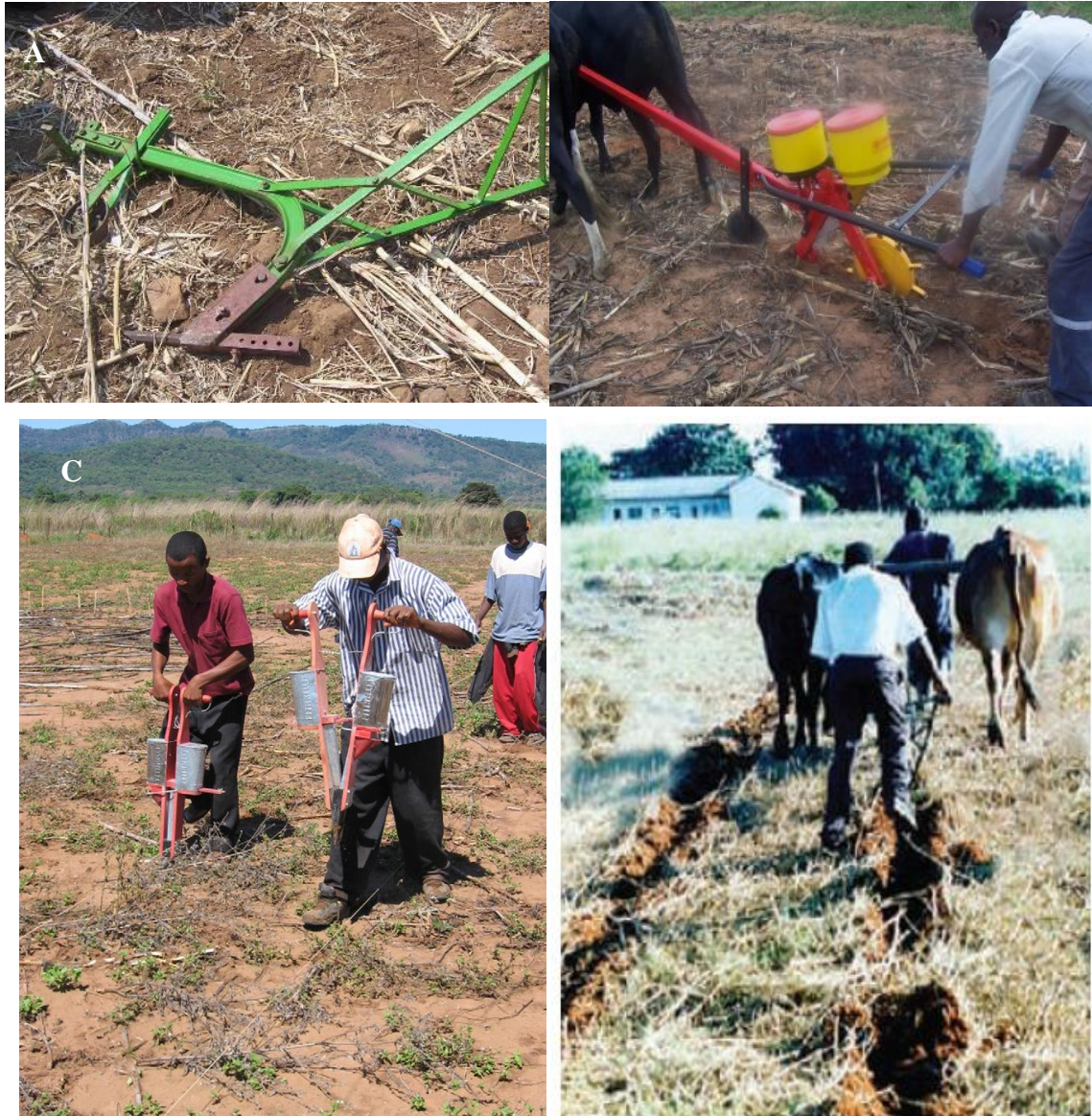
Figure 2.5 Figures showing implements for SH sector A) Ripper tine B) Ox drawn planter C) Jab planter (Photograph by Thierfelder in Johansen et al. , 2012) D) Ripper lines made by a Ripper (Adapted from ZCATF, 2009)
