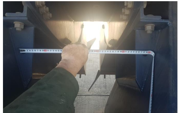
Figure 82 EDAQ bracket mounting location behind and between two buckets
