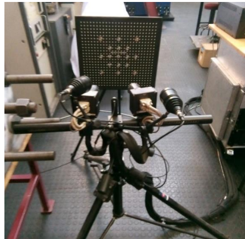
(b) Calibration setup with calibration panel placed 480mm from GOM cameras
