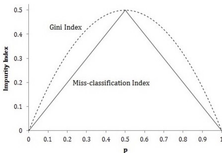
Figure 3.3: As per Hastie et al.[4] (p 309) showing node impurity measures for two-class classification being Miss-classification and Gini Index, as a function of the proportion p in the second class.
