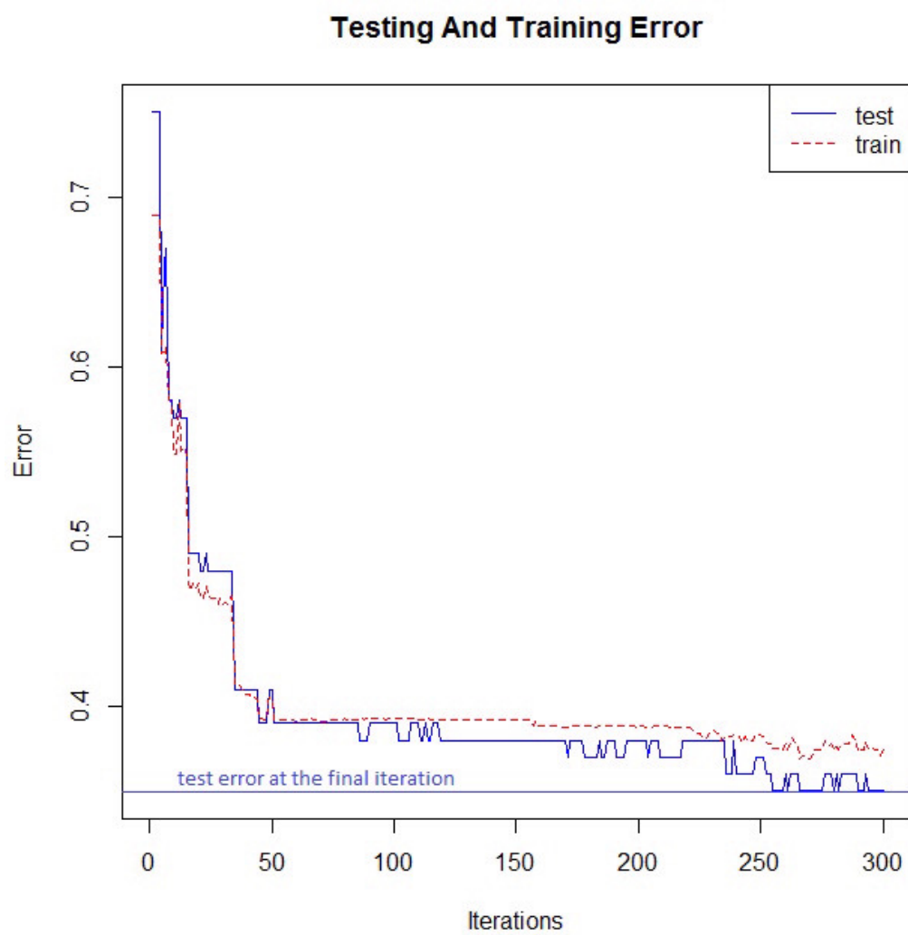
Figure 4.10: Graph showing the boosted training and test error rates using stumps based on simulated multi-classification data as per Section 3.5
