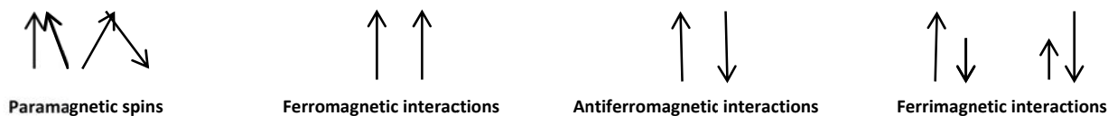
Scheme 1.6.2. The schematic representation of the possible spin interactions.
