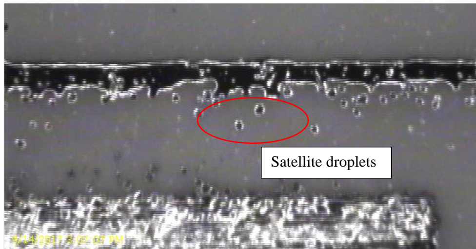
Figure 6.2. Fiducial camera image illustrating satellite droplets.
