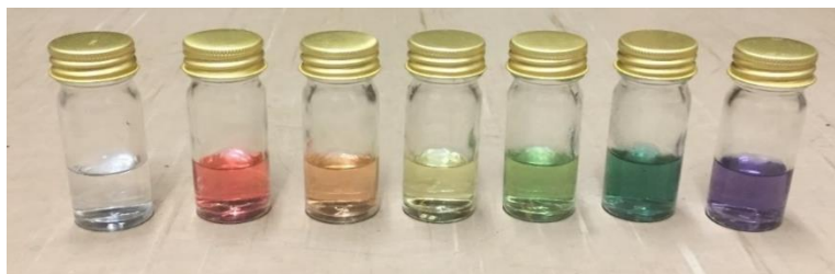
Figure 3.26. Liquid samples at different pH levels: Red (pH 4), Orange (pH 5), Yellow (pH 6), Light green (pH 7), Dark green (pH 8), Purple (pH 9).
