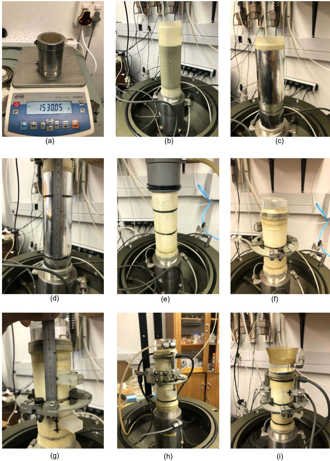
Figure 5-3: Sample setup procedure: (a) mass recording after reconstitution (b) sample placement on pedestal (c) wrapping of aluminium (d) measurement for local instrumentation (e) placement of O-rings on second latex membrane, (f) attachment of radial calliper and top cap (g) measurement of dimensions between vertical claps, (h) illustration of local instrumentation, (i) installation of suction sleeve
