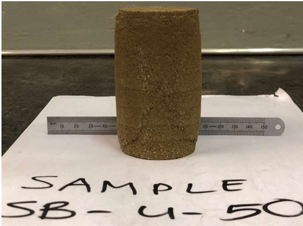
Figure 6-3: Failed sample of subballast material
