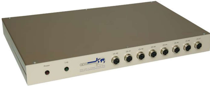
Figure 4-8: Serial data acquisition pad with 8 channels
