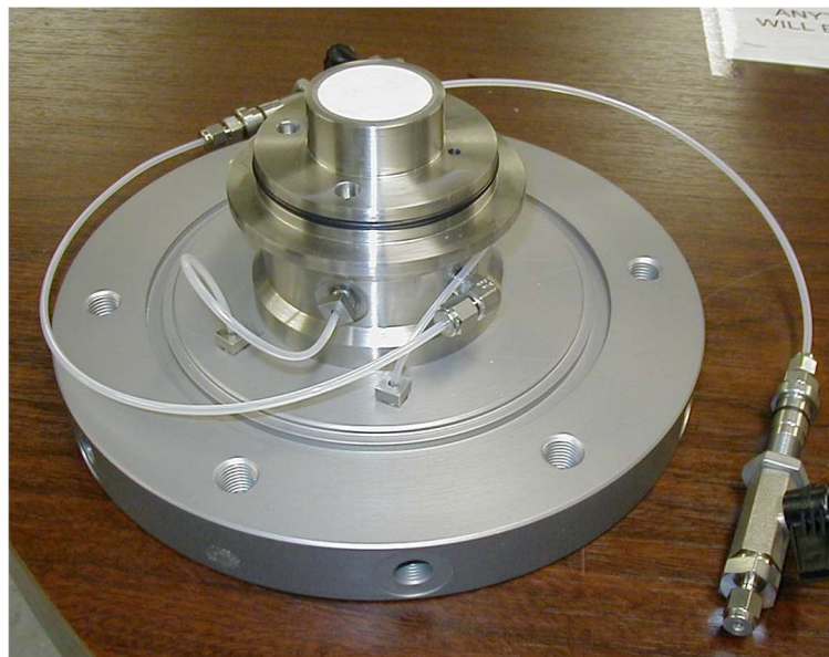
Figure 4-10: High air entry disk (Courtesy of GDS Instruments)
