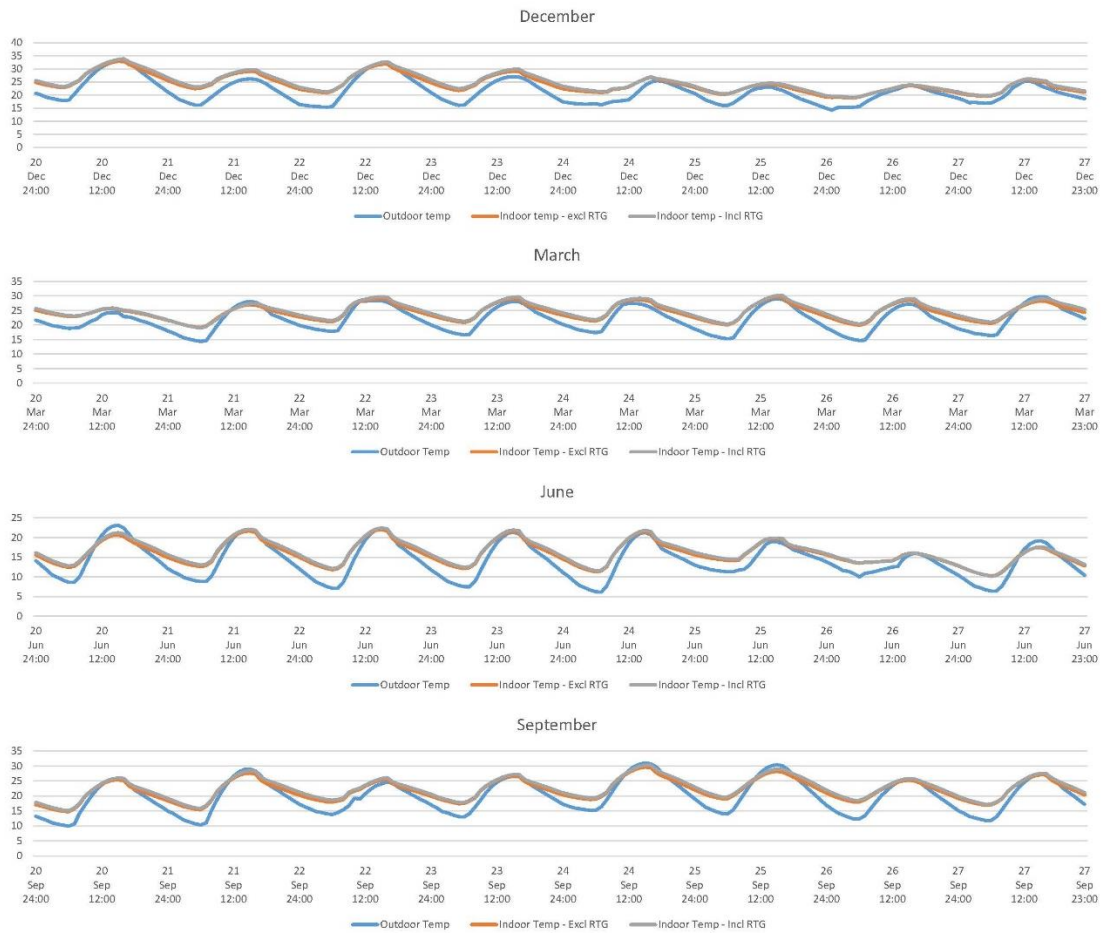
Figure 100: Temperature variations between models B1 (excl. RTGs) and B2 (incl. RTGs).
