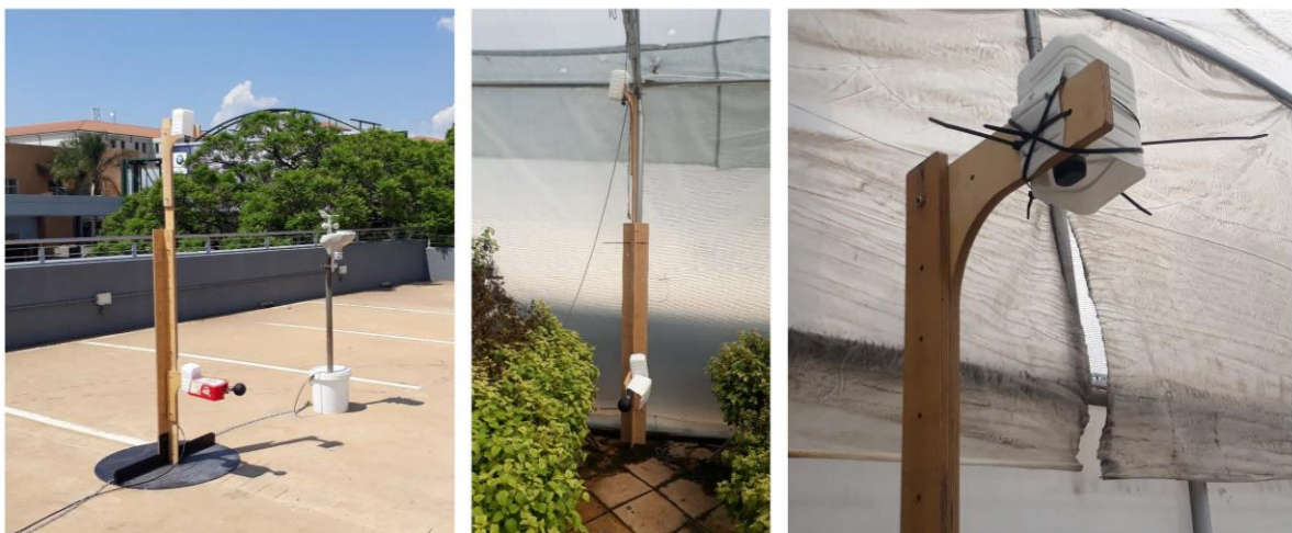
Figure 9: Typical location and installation of the sensors used to monitor the rooftop farms.
