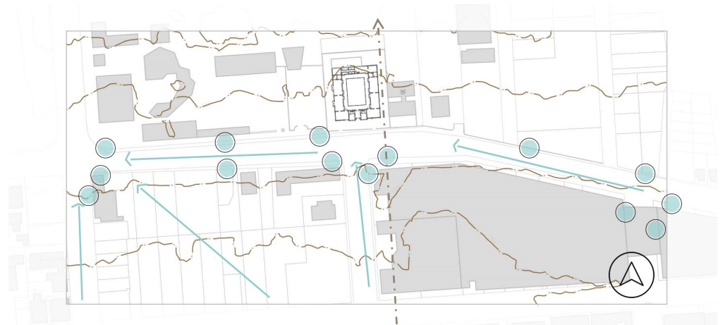
Fig. 2.17: Illustration of contours, the site slope and stormwater flow on impermeable surfaces into sewer systems (Author 2020)
