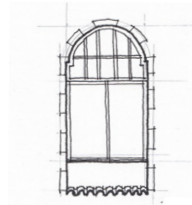
Double Side-Hung Window Old Stationary Storage Building
