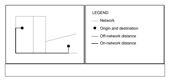
The distance (travel time or any impedance) between an origin and destination can be thought of as consisting of three parts (see figure 1): first an "off-network" distance from the origin location to a connection point on the network, second a "on-network" distance over the network from the origin's connection point to the destination's connection point and finally an "off-network" distance from the second connection point to the destination location.
