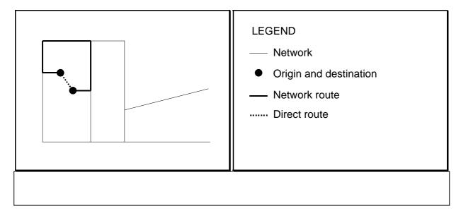
Finally we should consider if we need to use the network at all. It two data point are situated relatively close, it the optimal route might be a simple and straight "off road" connection between the two points (see figure 7). It can be argued that the direct route should at least be used, in case this connection is shorter than the two "off-road" parts of the normal route taken together.
