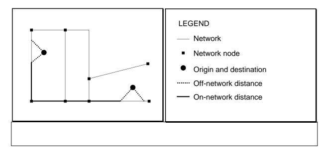
Thirdly we should consider the need to create more than one connection point per segment (see figure 6). In case a connection point is used the shortest path will always use only a part of the segment; either the part from start node to connection point or the part from end node to connection point. Especially when a road segment is curved the optimum connection point can differ dramatically between these two cases.
