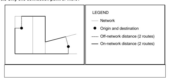
Once we've admitted the possibility of transport outside the digitised network model, the question must be asked: which other possibilities are there? Is it reasonable to assume, that there is one and only one transport link from each data point to the network, reaching that network at the nearest location? Or are there links in the opposite direction also, to another network segment located further away? Figure 3 illustrates a situation with two links from each data point.
