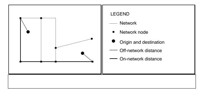
Evidently, if all the points of entry as defined above are represented in the network file as nodes, data points should be connected to nodes only (see figure 2). For example in our public transport study, we made all bus stops nodes by definition. The question is, what to do if this is not the case.
