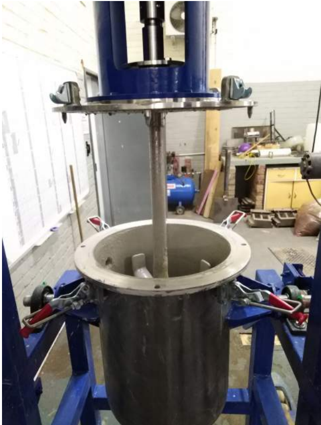
Figure C.2: Shear Mixer used to manufacture the artificial rock material.
