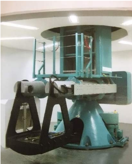
Figure C.1: Geotechnical Centrifuge at the University of Pretoria
