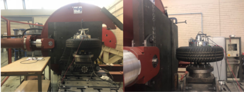
Figure 4.2: STTR in longitudinal and vertical loading position with smooth treaded tyre installed
