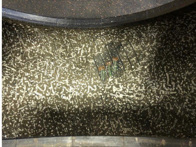
Figure 5.7: Installed inner surface strain gauges
