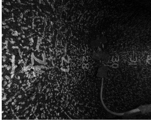
Figure 6.7: Inner surface strain gauges where silicon and lead wires can be seen to obscure the view of the installed region
