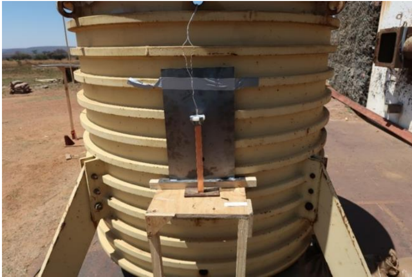
Figure 4.11: Setup of the copper tube against “vlip” wall
