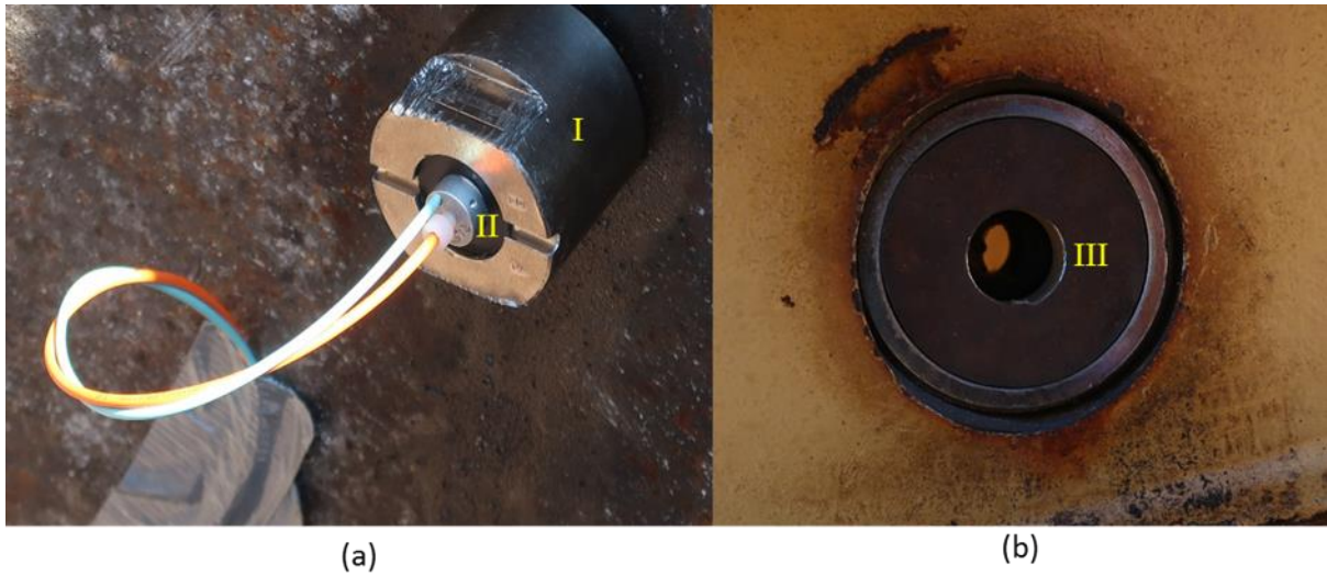
Figure 4.8: (a) Optical probe assembly inside the "vlip" showing the metal cylinder confining other components I and an optical probe II , (b) Optical probe assembly on opposite side of the "vlip" wall, showing the mild steel disc in front of the BK 7 window III.
