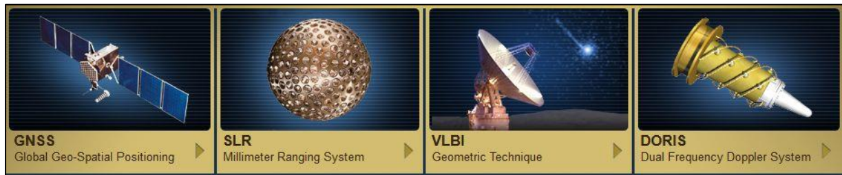
Figure 1. An illustration of the four main space geodetic techniques. The illustration represents a generic GNSS satellite, although in reality they are of different shapes and sizes; SLR's geodetic satellites like LAser GEOdynamics Satellite (LAGEOS) are spherical; VLBI relies on Earth based parabolic dishes; DORIS has dedicated antennas on ground stations. Source: NASA, 2018.
