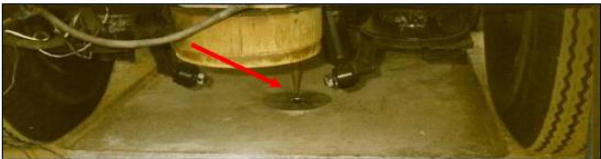
Figure 15. A stainless steel plate as a ground mark directly above the MOBLAS 6 telescope at HartRAO. The red arrow points to the SRP. Source: HartRAO, 2018.
