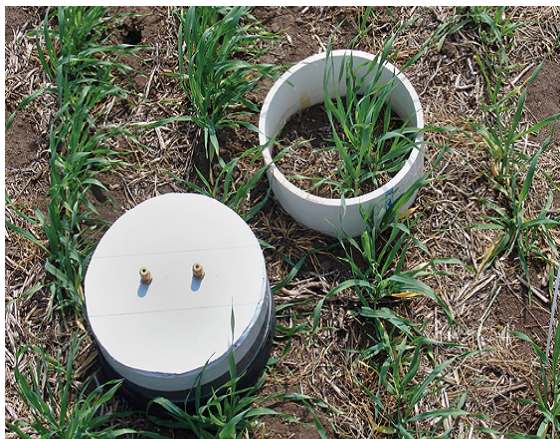
Figure 5 A static flux chamber head and base (Online: Chamber Picture, https://3c1703fe8d.site.internapcdn.net/newman/gfx/news/hires/2013/2-1-battlingclim.jpg , accessed 10 Feb. 2017)
