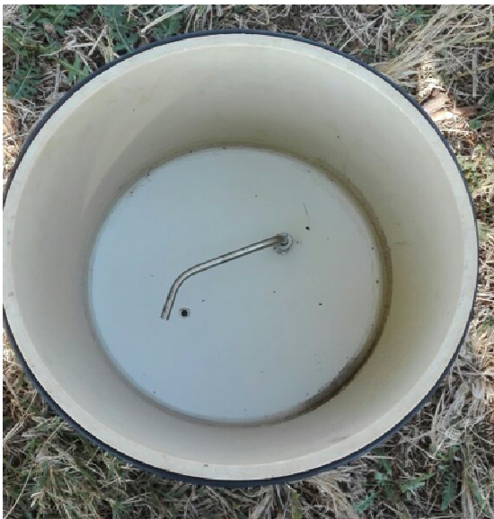
Figure 12 Underneath the closed static chamber head displaying the air vent
