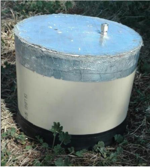
Figure 10 Closed static chamber head with injection port and reflective tape
