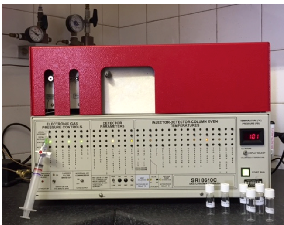
Figure 14 Gas chromatograph instrument at the University of Pretoria with 5ml vacuumed vials in front of the gas chromatography at the bottom right
