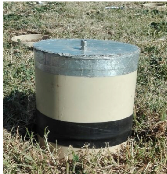
Figure 13 A joined closed static chamber head and base making up the closed gas chamber for gas collection
