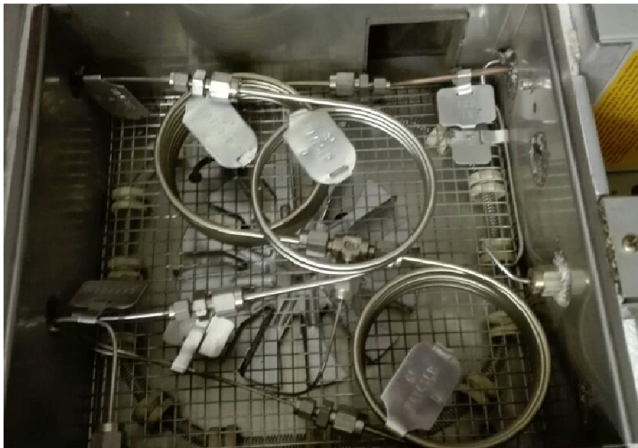
Figure 16 Displaying the HayeSep D packed stainless steel columns in the gas chromatograph instrument
