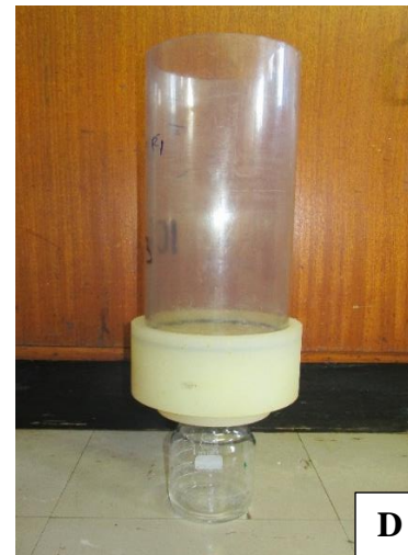
(A) Transparent Plexiglas column (length: 30 cm, internal diameter: 10.5 cm). (B) The five-layered mesh placed at the base of the column. (C) The depth filter secured on the column base. (D) the Plexiglas at the column base with the Schott bottle attached.
