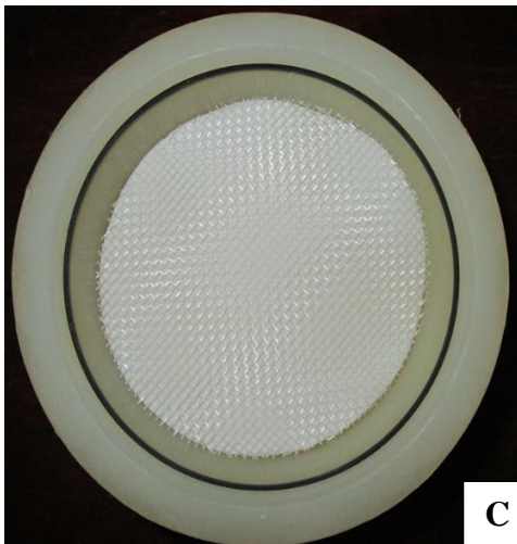
(A) Transparent Plexiglas column (length: 30 cm, internal diameter: 10.5 cm). (B) The five-layered mesh placed at the base of the column. (C) The depth filter secured on the column base. (D) the Plexiglas at the column base with the Schott bottle attached.
