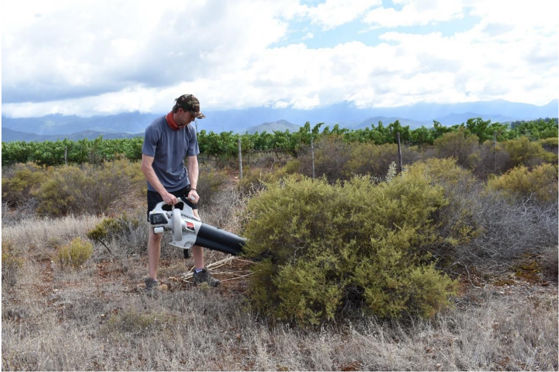
Figure A.3: Suction device which consisted of a leaf blower (set to suck the air in, instead of blowing air out) and attaching a stocking to the front of the leaf blower with an elastic band to collect the insects inhabiting the plants sampled. The device was used for 10 seconds to collect insects from small plants, 30 seconds for plants larger than 30 cm, and 90 seconds for plants larger than 1 meter in size.
