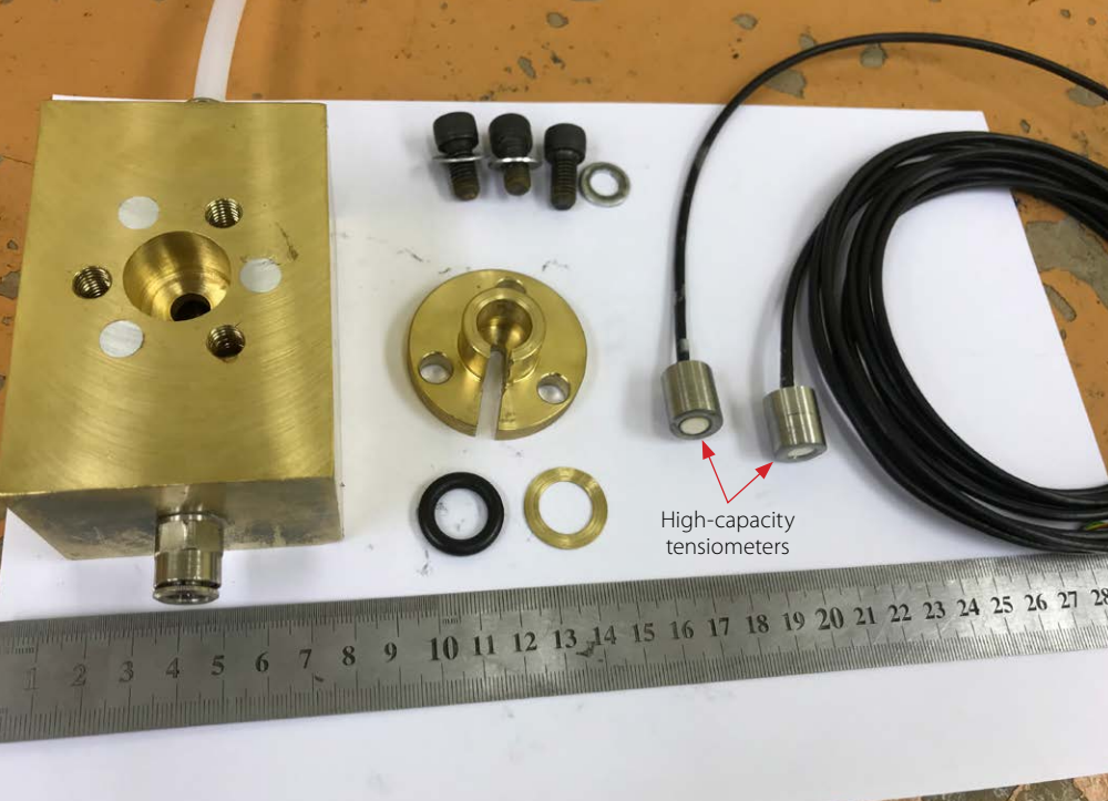
Figure 3 Two new high-capacity tensiometers and the saturation equipment
