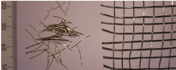
Figure 5.2 Micro-steel fibres and prepared mesh
