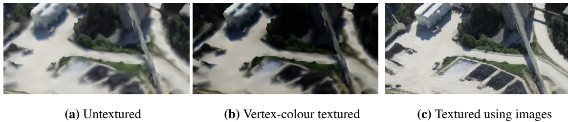
Figure 3.7. The third comparison of textures generated from the mesh’s vertex-colours and textures generated from the original images, using meshes generated from the Swiss quarry dataset [36].
