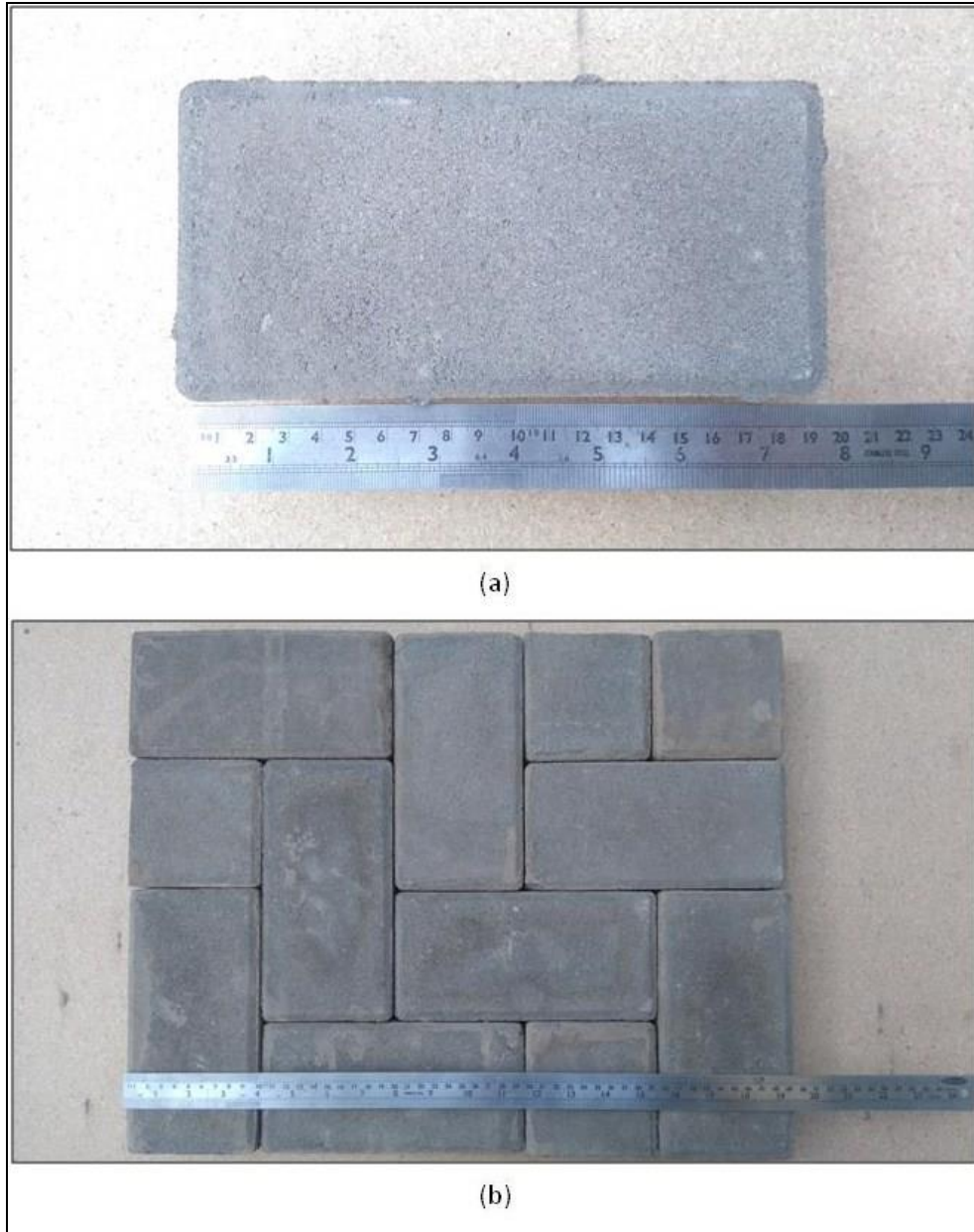
Fig. 16: (a) The selected brick paving unit, Product 55: Bevelled and (b) the selected arrangement of bricks for the surface layer. (Supplied by MVA Bricks Pta. West)
