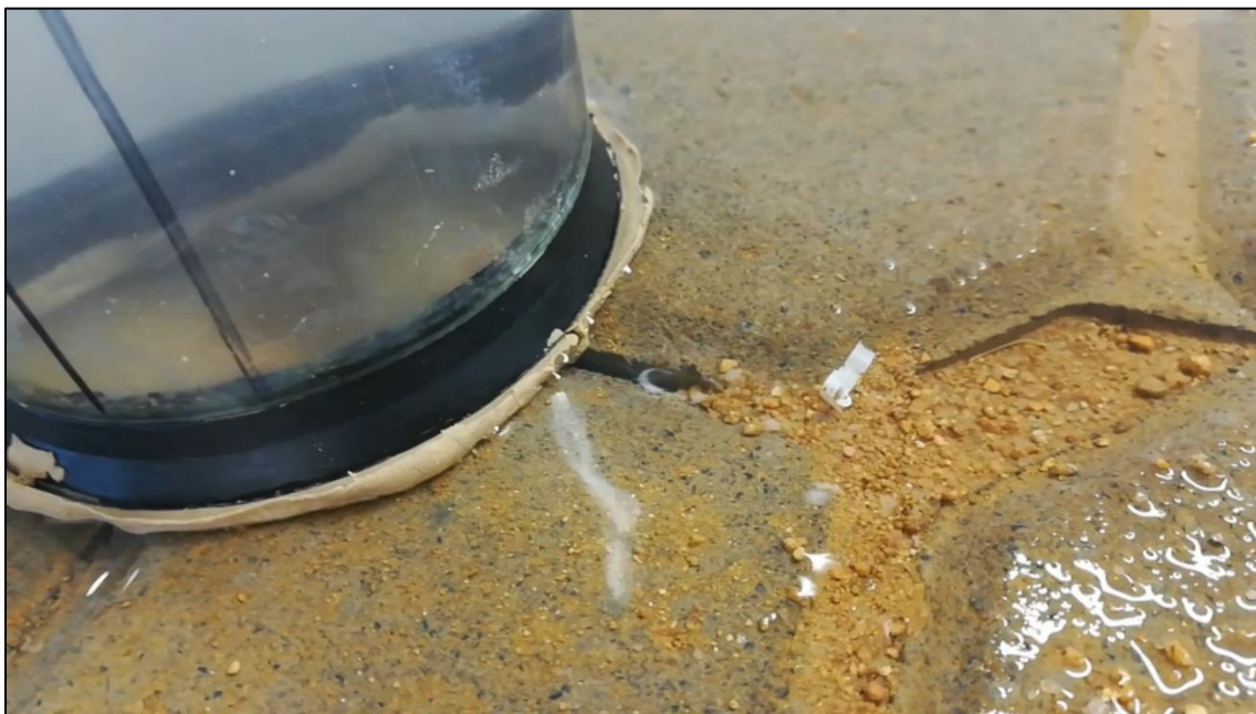
Fig. 41: The erosion of jointing material beneath the sealant of the inner ring of the double-ring infiltrometer constructed for this study
