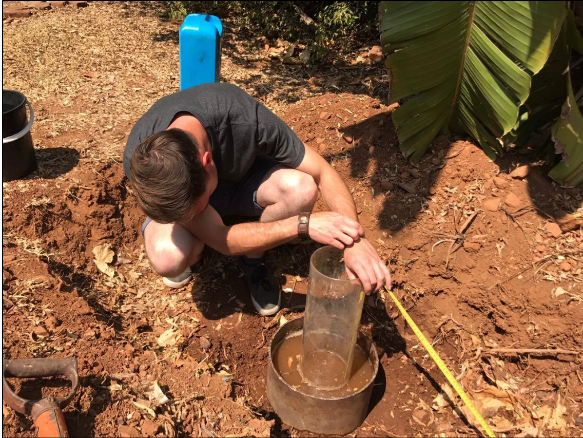
Fig. 8: The Double-Ring Infiltrometer constructed for field tests conducted on the Brooks St. site.
