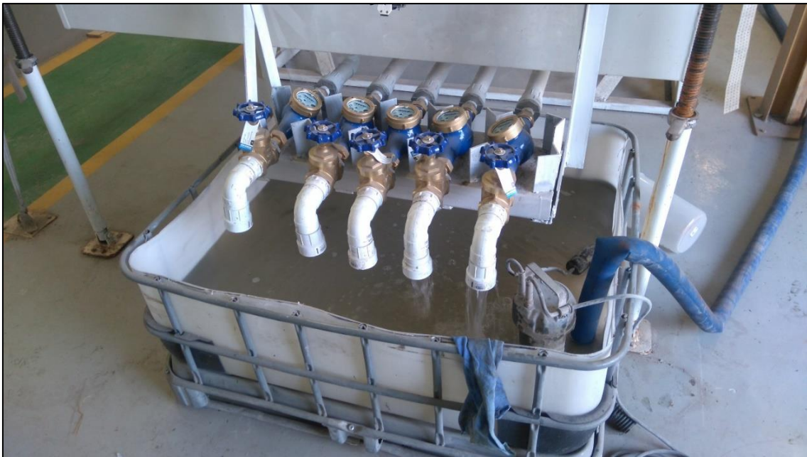
Fig. 14: The outlet system of the Infiltration Table Apparatus (Bosun – Midrand, 2019).
