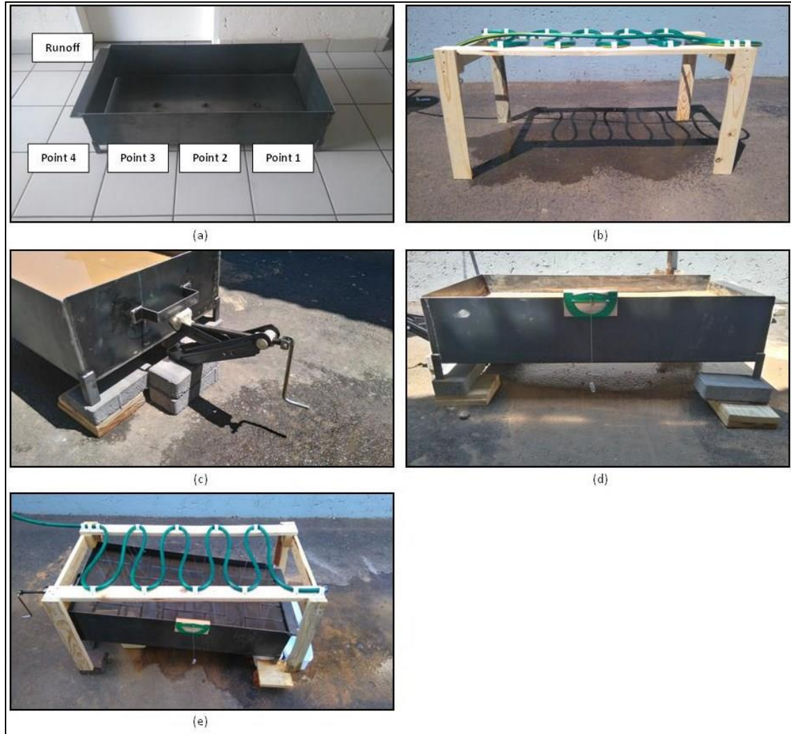
Fig. 10: The apparatus constructed to perform tests on the representative volume for the basic flow model.
