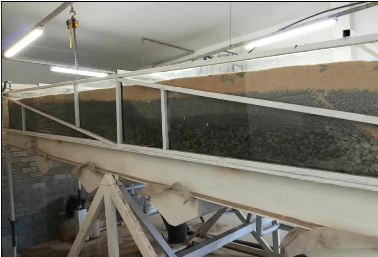
Fig. B-6: An image showing the side view of a completed construction of a Citylock® and P-Type 1 sand containing layer works in the Full-scale Model shortly before testing. Here, the filter media can be seen in the collection bins below the ITA and the block and tackle used to change the incline above.
