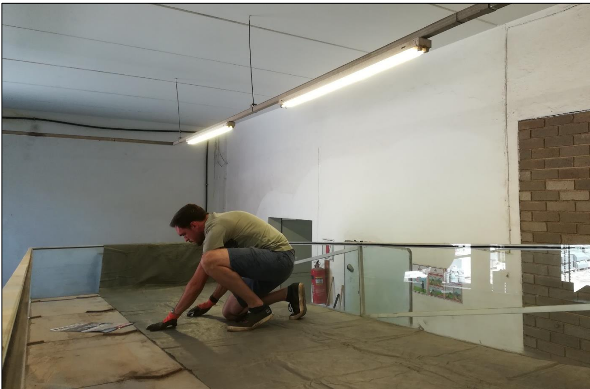
Fig. B-2: An image of the bibum being cut to size for use in the Full-scale Model Testing.
