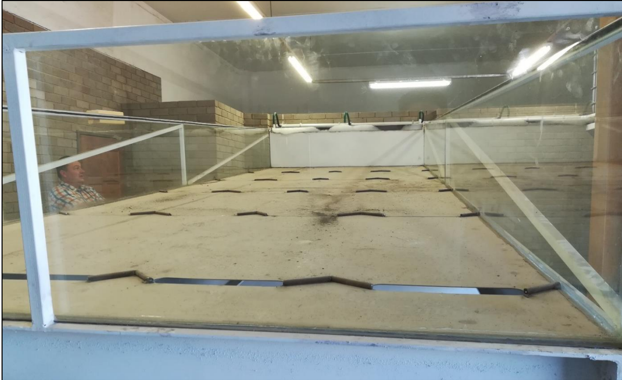
Fig. B-1: An image of the Infiltration Table Apparatus showing the guide rods welded to the construction surface (deck).
