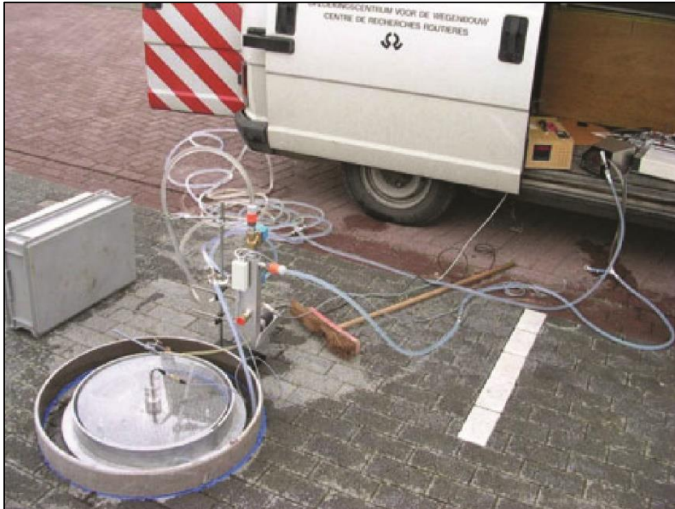
Fig. 7: A Double-ring Infiltrometer Test modified for use on ICP.
