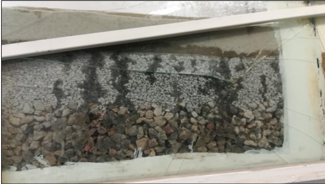
Fig. 39: Tendrils formed in the sub-base layers for Full-scale Model testing of a layer works containing a Citylock® and P-Type 3 sand surface combination at an incline of 2.5°
