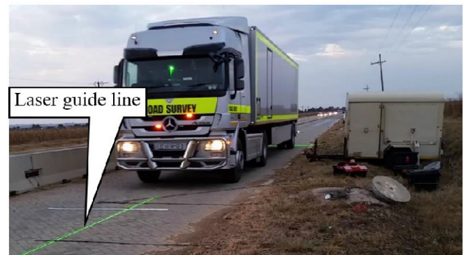
Fig. 3. SANRAL Traffic speed deflectometer truck on test section.
