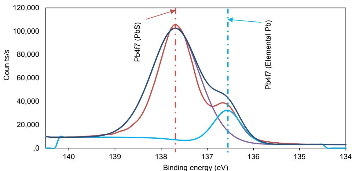
Figure 6: XPS Pb narrow-scans for the film formed for a Pb(II) concentration of 100,000 ppm.
