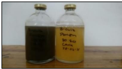
Figure 2: 80 ppm Pb(II) & 40 ppm Zn(II) on the left versus 80 ppm Pb(II) & 80 ppm Zn(II) on the right.
