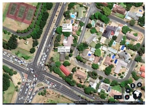
Figure 1: Typical road layout showing hard shoulder and turning lane (this example taken from Site 2), Google Earth 2019.
