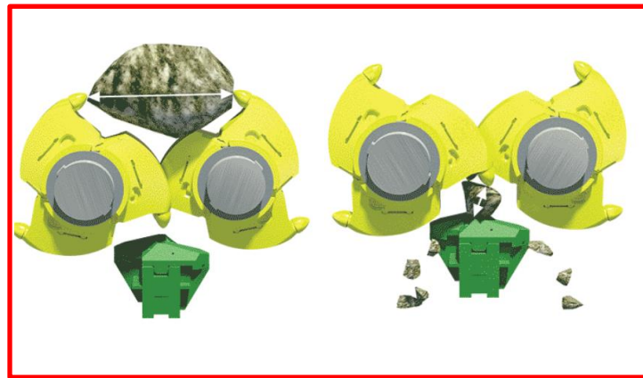
Figure 20 : Operations principle of the mineral sizer
