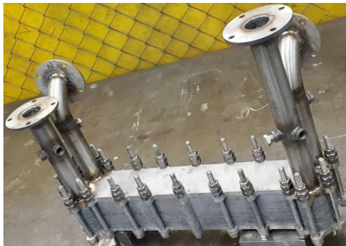
Figure 24 Assembled Mark II core.
