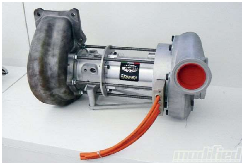
Figure 8 Magneti Marelli TERS turbocharger (Formula 1 Dictionary, 2014).
