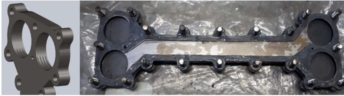
Figure 20 SolidWorks Mark I recuperator model (left); experimental model being assembled with Calofer (right).
