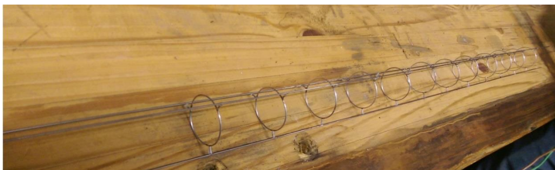
Figure 15: Final turbulators manufactured.
