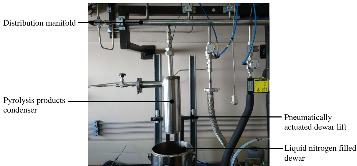
Figure 3: Annotated photograph of the pyrolysis gas condenser system
