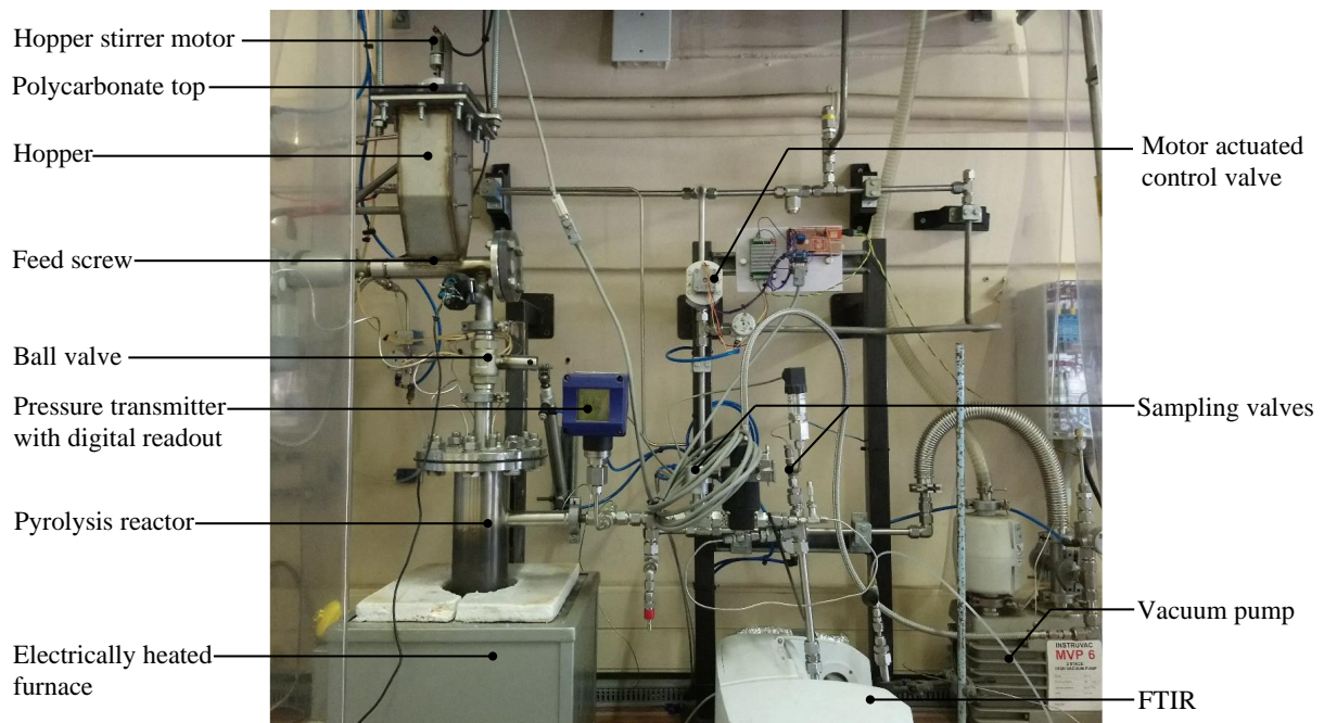
Figure 1: Annotated photograph of the pyrolysis reactor set-up
