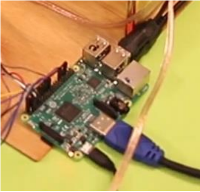
Figure 8-12 Raspberry Pi as physical IoT device
