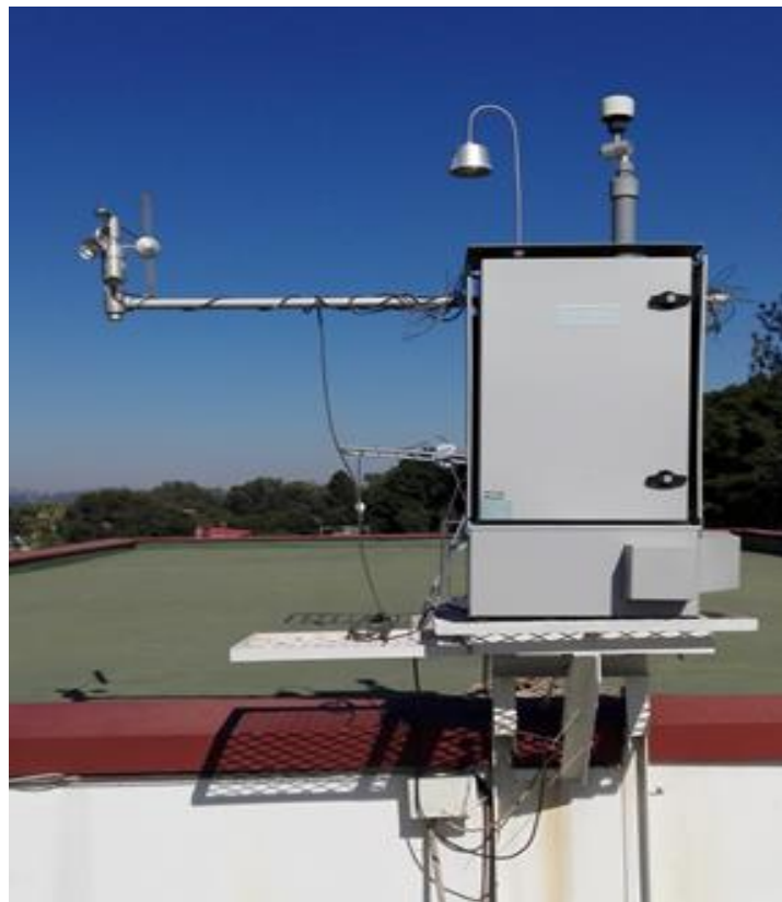
Figure 3.6: Image of Aeroqual instrument on the roof of the HW Snyman South building, University of Pretoria
