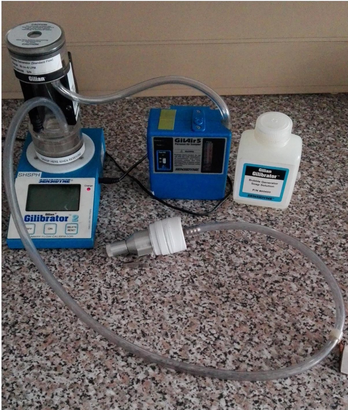
Figure 3.3: GilAir pump connected to the calibration unit
