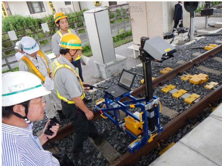
Figure 2-1: The current measurement system used in Japanese train stations (Shimizu, 2016)
