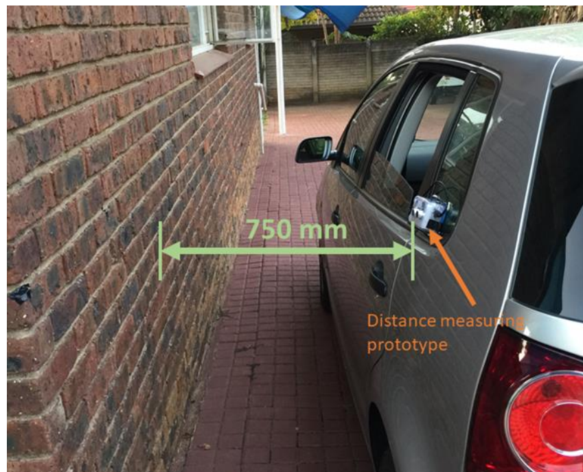
Figure 3-16: Experimental setup depicting measurements recorded at a distance of 750 mm
