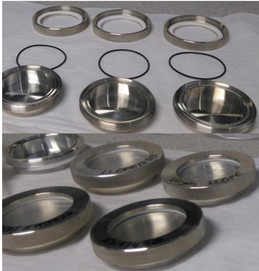
Figure 3.3: Payne permeability cups, rings and polymer nanocomposite films used to study the permeability of the repellents through polymer film
