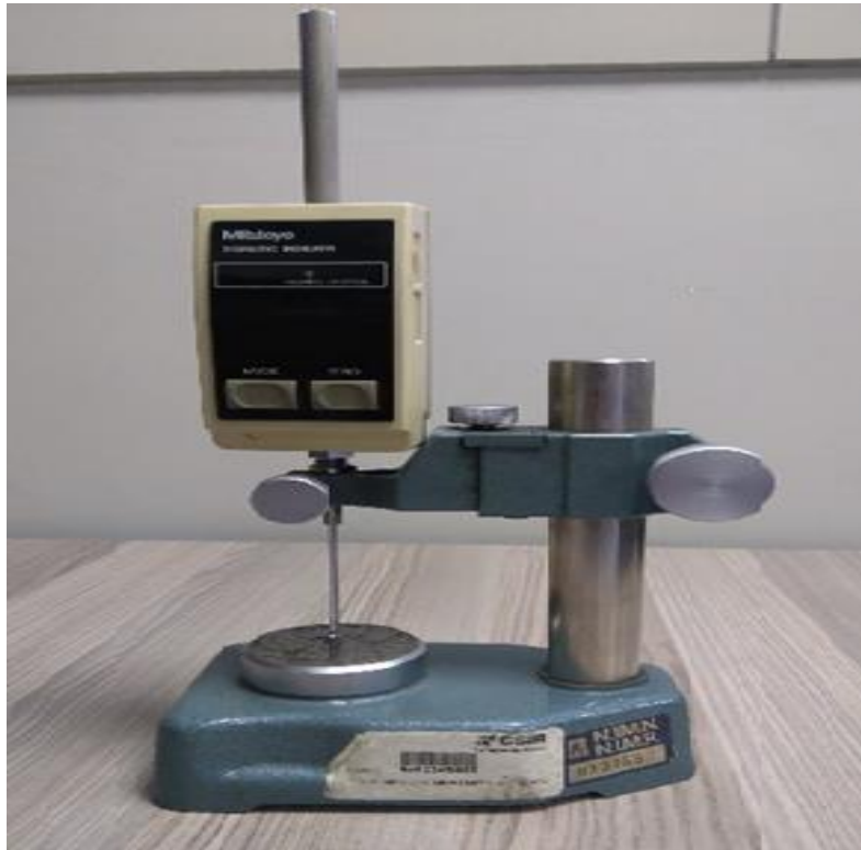
Figure 3.2: Thickness measurement using a Mitutoyo Digital micrometer
