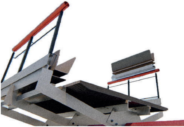
Figure-170: Step 9- Placement of pre-manufactured lightweight concrete planters and drip trays.
