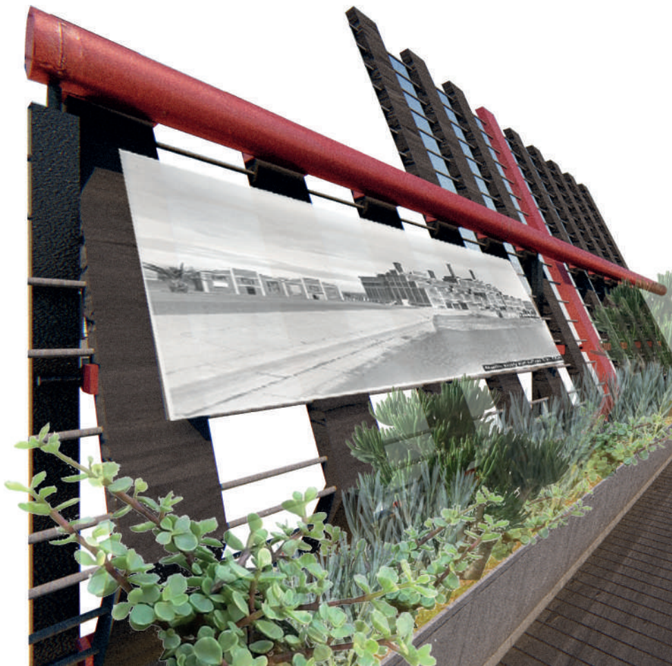
Figure-157: Perspective views of the high balustrades and photo frame details along initial section of the Carbon Skywalk.
