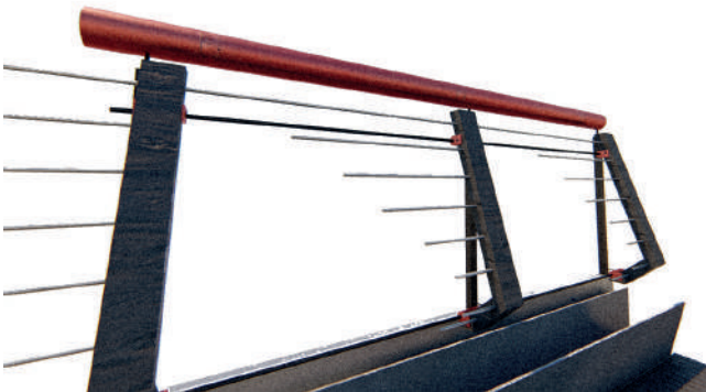
Figure-172: Step 11- Threading of galvanised steel rope through pre-drilled holes in the balustrade posts.
