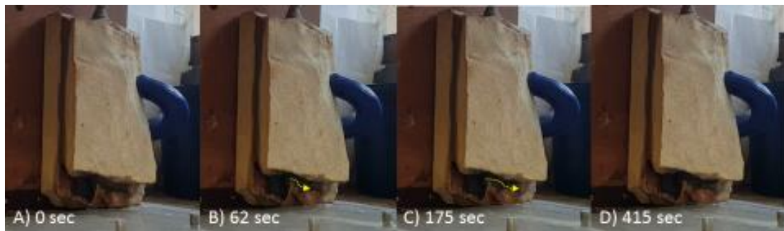
Figure 4-9: (A-D) Flow pattern in shale for the wet and rewetting phase inclined at 90°.
