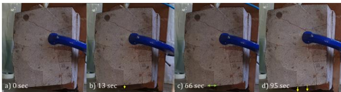
Figure 4-16: (a-d) Flow patterns in quartzite for the initially dry phase inclined at 90°.
