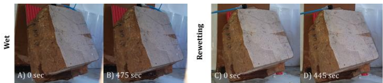
Figure 4-15: Flow pattern in quartzite for the (A-B) wet and (C-D) rewetting phase inclined at 60°.
