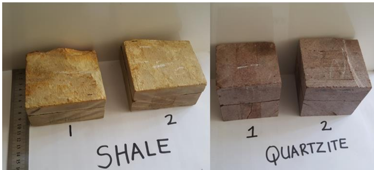
Figure 3-6: Shale and quartzite samples sawn to dimensions of 100mm × 100mm.
