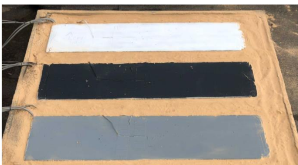
a) Concrete beams after application of paint
