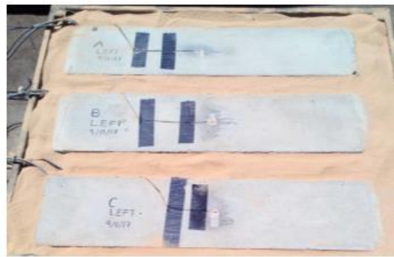
d) Concrete beams fully embedded in sand
