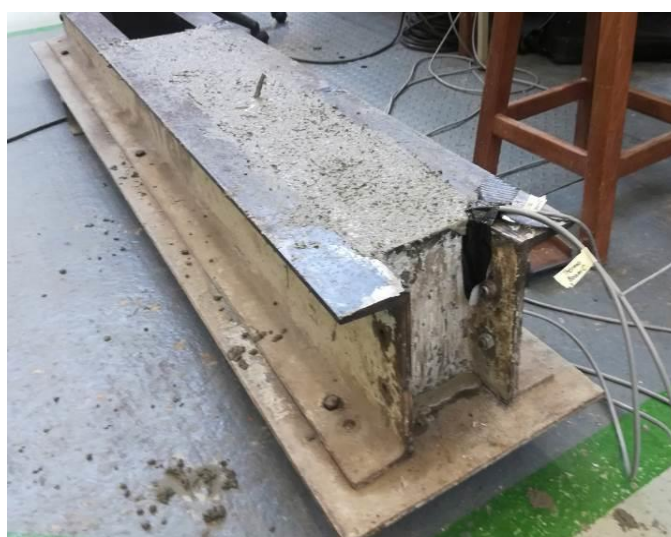
Figure 3-2: Concrete beam immediate after placement of concrete.
