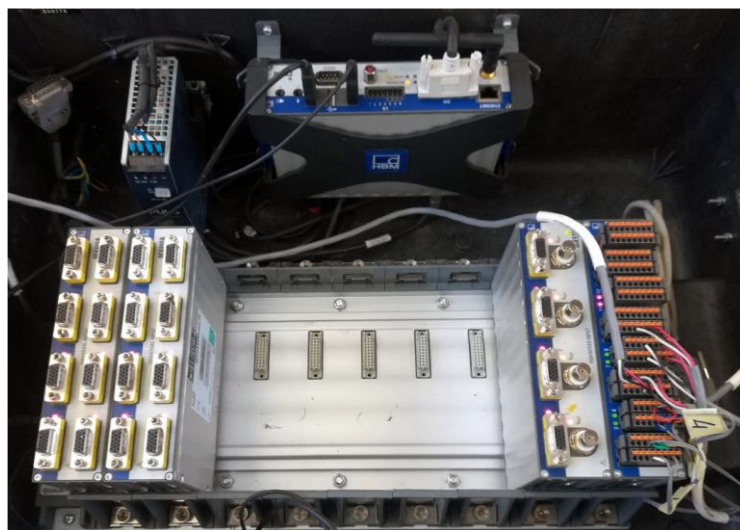
Figure 3-12: HBM QuantumX universal amplifiers.
