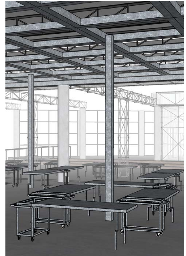
Figure 6.6.2.9 - Digital visualization of market infrastructure, trader trolley, trestle table and service column (Author, 2019)
