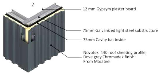
Fig.59: Sheet metal and LSF wall construction (Original image. Archello, 2019)
