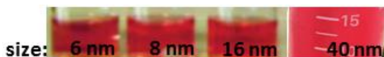
Figure 4.3: Bright red colour of differently sized colloidal gold nanoparticle suspensions. From Ojea-Jiménez and Puentes 149 and own image (40 nm).
