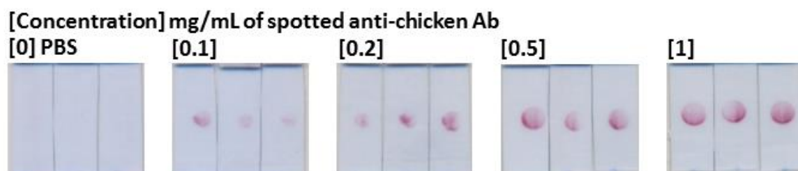
Figure 4.12: LFTs comparing the signal intensity of gold labelled gallibody conjugate at a concentration range of immobilised anti-chicken IgG (Fc) antibodies. Increasing concentrations of goat anti-chicken IgG (Fc) antibody in PBS were coated on the nitrocellulose and probed using gold labelled gallibody 18-2 conjugate (at 0.04 mg/mL to OD 1 gold at pH 6) in the LFT format. A flatbed scanner was used to image the test results. Test sections shown were cropped from a single image.
