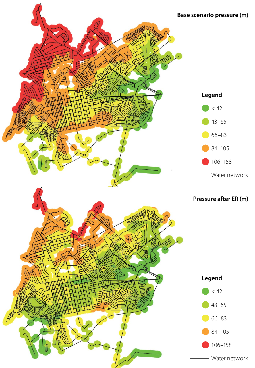
Figure 6 Polokwane Central DMA operating pressure distribution before and after energy recovery
