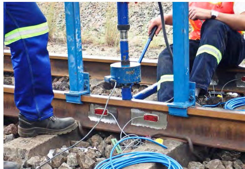
Figure 1 Typical strain gauge setup for wheel load measurement with a calibration frame positioned between two sleepers
