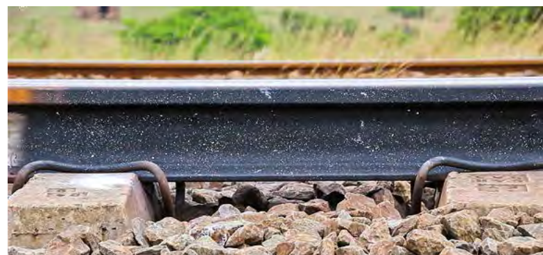
Figure 2 Typical field setup using PIV where the rail is painted with black paint first and then with a random spray of white speckles
