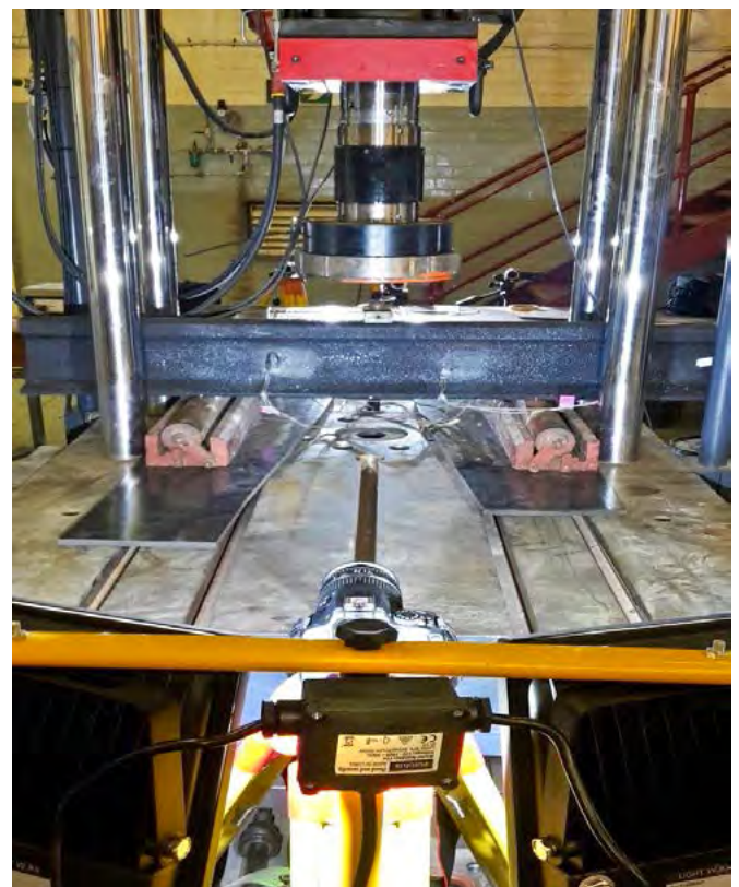
Figure 4 LED lights were set up behind the camera to improve the image quality of the rail surface
