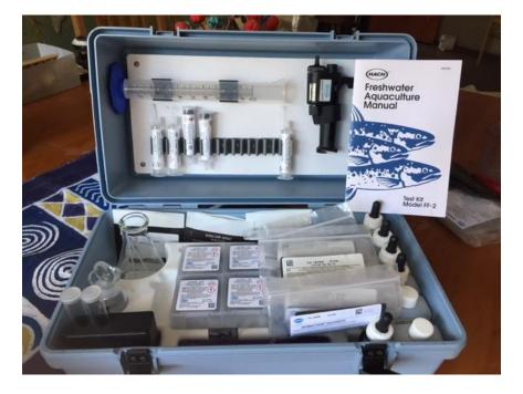
Fig. 3-1 HACH Model FF2: Fish farming freshwater test kit
