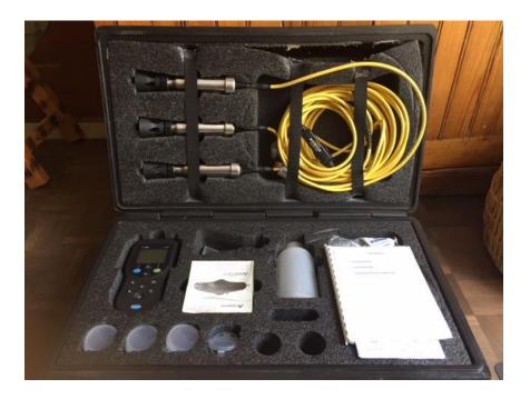
Fig. 3-2 HACH<sup>®</sup> HQd IntelliCAL Rugged field kit
