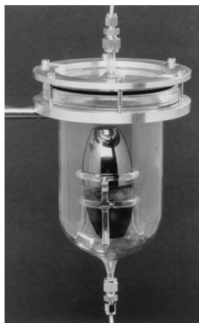
Figure 2-9: Sublimation setup used for the purification of ZrF_4
