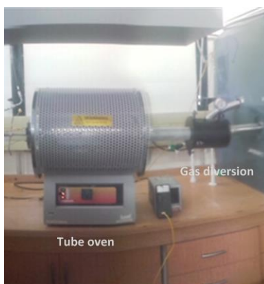
Figure 3-5: Illustration of the sublimation/desublimation setup
