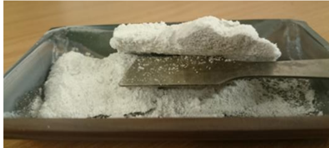
Figure 6-2: Sublimation residue indicating cake formation
