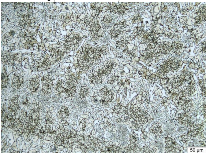
1100 °C +FAQ + 350 °C T (etched with Le Pera)
