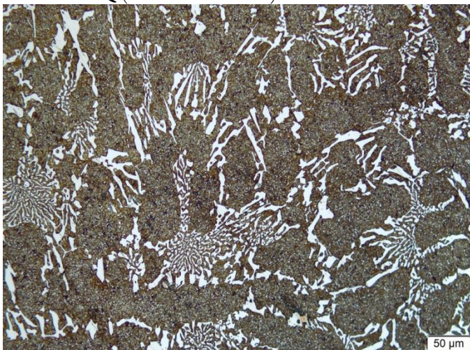
1050 °C +FAQ + 350 °C T (etched with Le Pera)
