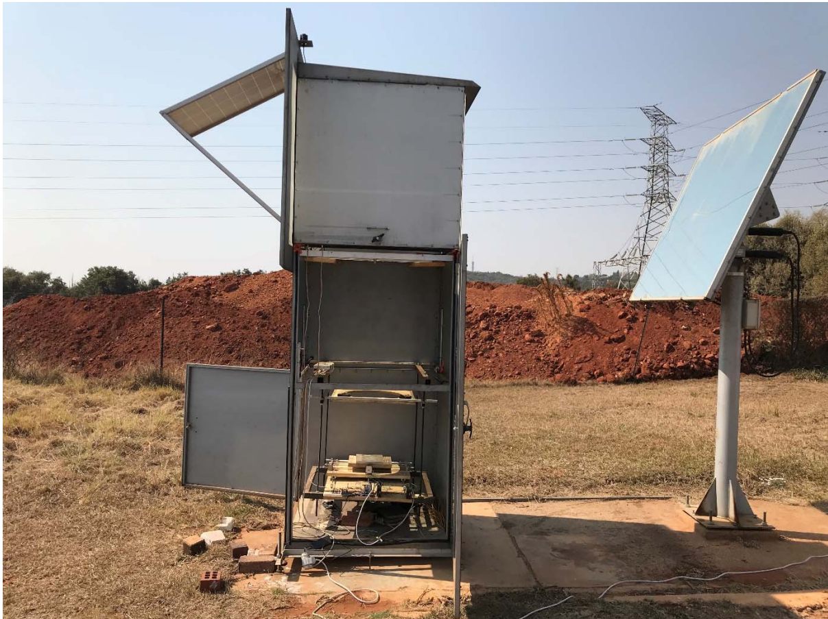
Figure 4.4: Constructed 3D Printer Mounted in Concentrating Platform
